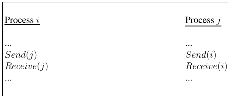
Figure 6.4: A communication program for an asynchronous system deadlocks when using synchronous primitives.
