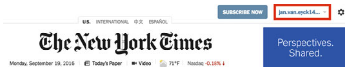
Fig. 3 The email address of a logged-in New York Times user is displayed on the top banner of the website (highlighted in red). Because the New York Times does not deliver their webpage over an encrypted connection (as of September 2016), an eavesdropper can use the email address to assign a real-world identity to a pseudonymous web browser
