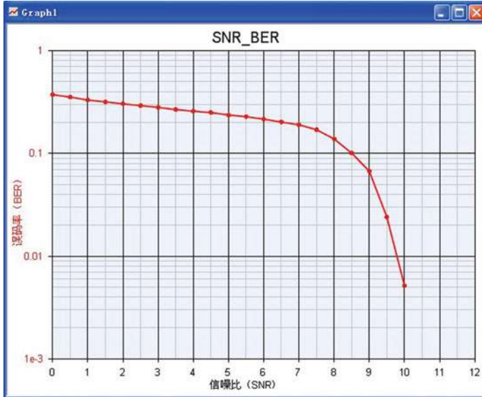
Fig. 5.21 CDD-OFDM system BER simulation test results
