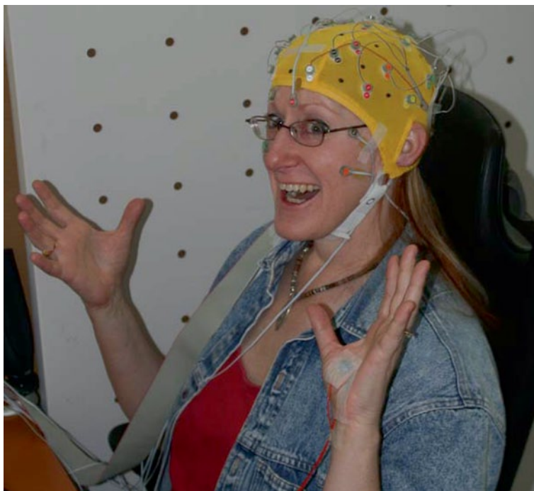
Fig. 4.3 EEG, EMG, and GSR electrode setup shown on a study participant
