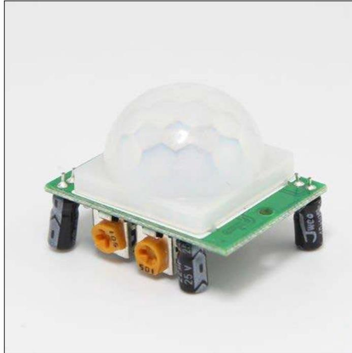
For the motion detection, we'll be using a generic HC-SR501 **Passive Infrared (PIR)** motion sensor supporting 5 V. This type of sensor can detect motion by measuring heat changes in its surroundings.
