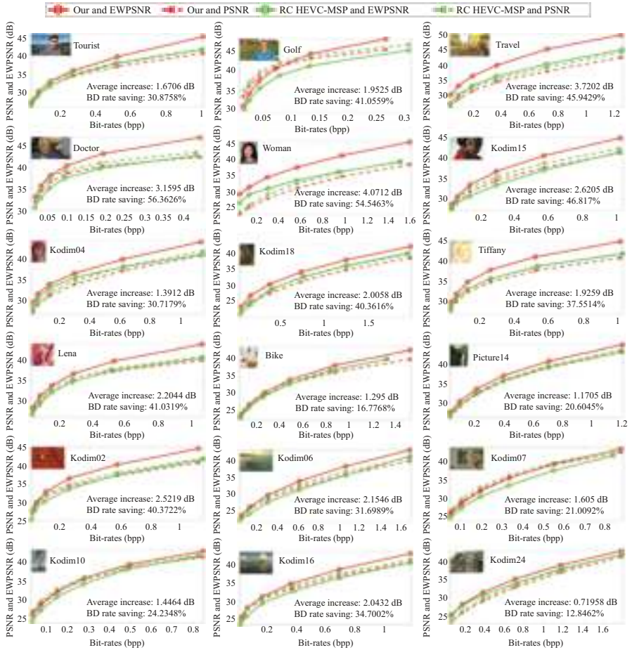
Figure 8.6 EWPSNR and PSNR versus bit rates for our approach and the RC HEVC-MSP [11]
