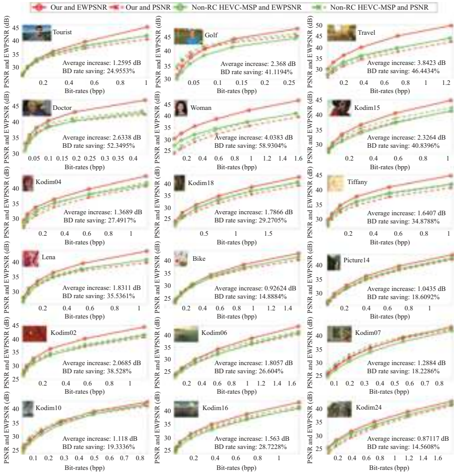
Figure 8.5 EWPSNR and PSNR versus bit rates for our approach and the non-RC HEVC-MSP [11]
